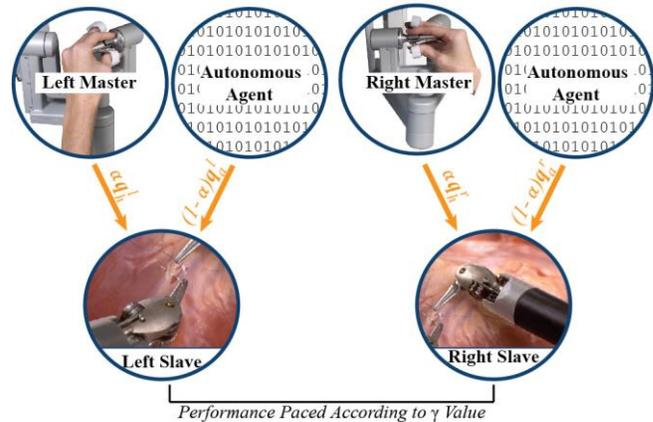
Fig. 1. Schematic of the shared-control architecture. Authority over the slave robots is arbitrated between the left and right master tool manipulators and an autonomous agent. The authority of the human operator and autonomous agent is defined according to the dominance factor ( $\alpha$ ) and the performance pace is defined according to the aggressiveness factor ( $\gamma$ ). Images ©2015 Intuitive Surgical, Inc.
