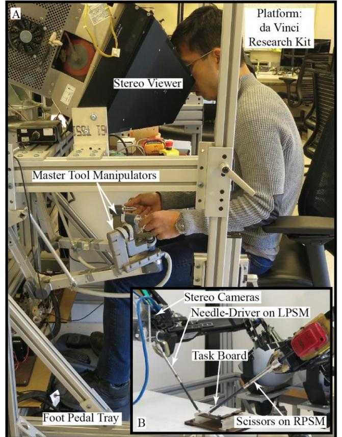
Fig. 2. The da Vinci Research Kit was used as the experimental platform. A: The participants were seated at the master side and used master tool manipulators, foot pedals, and stereo viewer, B: A needle driver and curved scissors were used on the left and right patient-side manipulators, respectively.
