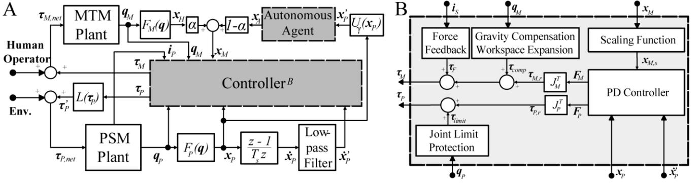
Fig. 3. Block diagram of the implementation of the architecture on the da Vinci Research Kit. A: General control structure, B: Controller design.
